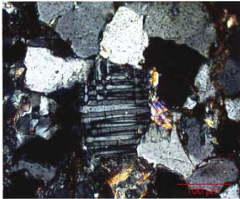
Figure 6.4. Microphotograph of a microcline (perthite), quartz grains and some calcite cement. Note grain-supported fabric. From the Stubdal Formation, quarry near Utvika (locality RG30) (in cross-polarized light).
